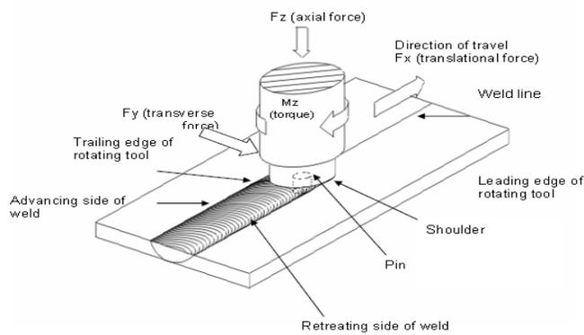
**Fig. 1 Schematic of the FSW Process [Kumar et al., 2011]**
