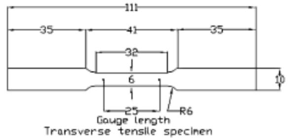
**Fig. 4. Transverse Tensile Specimen**
