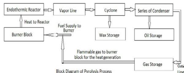
Fig. 2:- Block Diagram of Pyrolysis Process
