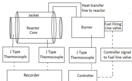
Fig. 4:- Temperature control for reactor - working diagram
