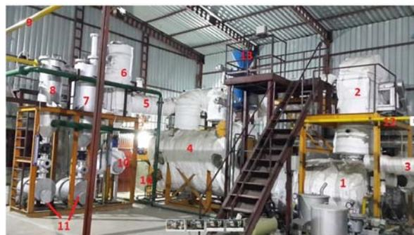
(1- Burner block, 2- ID fan, 3- FD to burner block line, 4- Endothermic reactor, 5- Vapor Line, 6- Cyclone, 7 & 8- Condensers series, 9- Gas line to gas storage, 10- Wax collection tank, 11- Oil collection tanks, 12- Gas line from gas storage to burner for firing, 13- Feeding hopper, 14- Carbon screw)
